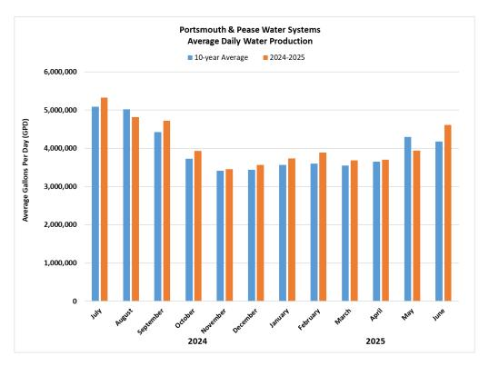
The following graphs illustrate the current Quarter's water production relative to the current supply capability for the Portsmouth and Pease Drinking Water System supply sources. Both systems are showing a good buffer of available supply versus demand. The current supply capability varies depending upon the conditions of the source including water levels and source water quality.
