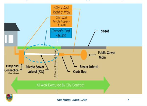
BLUE = HOMEOWNER COST: Private lateral sewer pipe ORANGE = CITY COST: Sewer pipe under the street, connection to lateral, pump and connection to house
